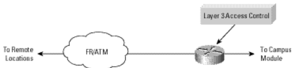
Figure 12 Attack Mitigation Roles for WAN Module
